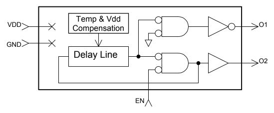
Figure 1: 3D7702 Functional Diagram
