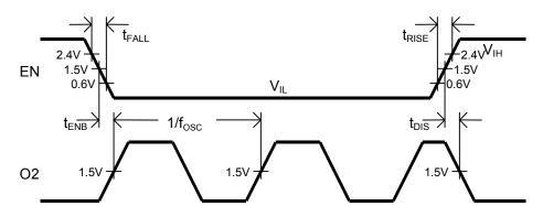
Figure 4: Timing Diagram
