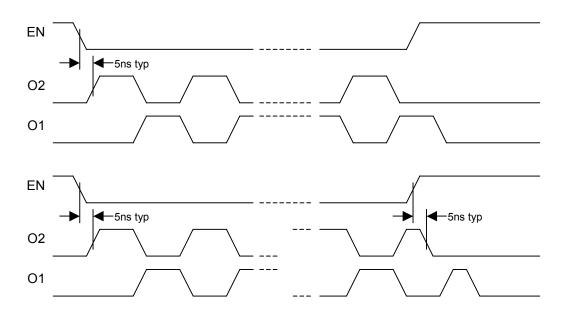
Figure 2: 3D7702 Timing Diagrams
